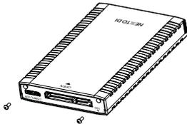
Close the aluminum case and tighten 2 screws on the connector side.
