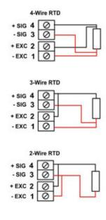
In 4-wire hookup, different pairs of leads are used to apply the excitation current and sense the voltage drop across the RTD, so that the IR drop across the excitation leads is not a factor.
