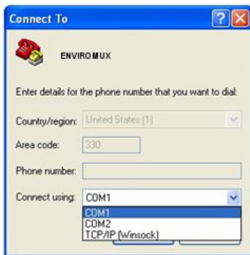
Figure 11- Configure COM port in HyperTerminal
