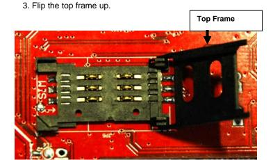
4. Insert the Mini SIM card into the slot on the top frame. The contacts should be facing you and the cut-off corner of the card should be towards the right. Insert the card all the way in until it stops.
