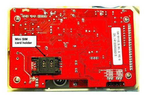
2. Slide the top of the card holder to the right. A gap will appear between the top and bottom of the cardholder.
