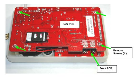
2. With the screws removed, carefully pull the rear circuit board off of the front circuit board. Lift the circuit board straight up to separate them.
