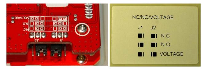
NOTE: The "VOLTAGE" jumper position is <u>not used</u> in conjunction with the ENVIROMUX-xD.
