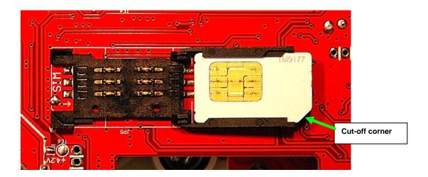
5. Fold the top frame back on top of the bottom. The card should set into the same-shaped recess in the bottom.
