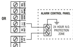
The Alarm Output switches to (-) ground in door forced to open or the door open after Egress Delay. You may use it to turn ON an LED lamp and/or a small buzzer to notify a guard; or connect it to a 24 hour Normally Open protection zone of an alarm system. See Location 80 and Location 91 for more information about these functions.
