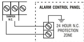
The tamper switch is Normally Closed while the keypad is secured on gang box. It is open when the keypad is removed from the gang box. To prevent sabotage, connect these terminals in series with a 24 hour N.C. protection zone of an alarm system if required.
