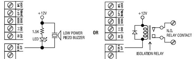
The Key Active Output switches to (-) ground for 10 seconds whenever a key is touched. You may use it to turn ON an LED lamp and for a small buzzer to notify a guard; or to energize a relay to switch ON lights or trigger an CCTV Camera to start recording.
