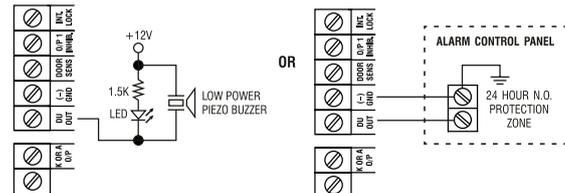
The Duress Output switches to (-) ground when duress code is entered. You may use it to turn ON an LED lamp and/ or a small buzzer to notify a guard; or connect it to a 24 hour Normally Open protection zone of an alarm system.
