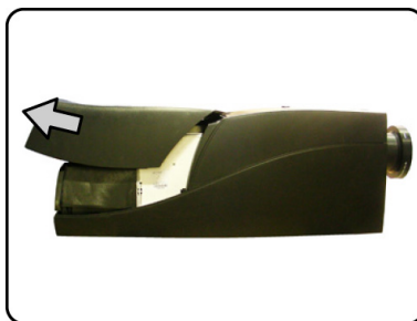
Image 3-3 Pull the rear cover backward
