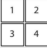
: Quad 2 x 2       | Four inputs are required. The sources are displayed in four quadrants.                                                        | Quad Combo input:<br><ul style="list-style-type: none"> <li>4x SDI input</li> </ul> Quad DP 1.2 Input:<br><ul style="list-style-type: none"> <li>4x DisplayPort</li> </ul>                                                        | Mono / Active stereo |
