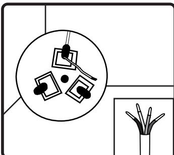
2. Locate speaker wire on the underside of the speaker. Strip wire ends if neccessary.
