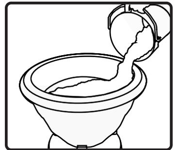
4. Place speaker in desired location. Fill planter with pea-gravel to approximately 2" above the black insert box to ensure proper drainage. Gently rock the planter from side to side so that gravel fills in the gaps, providing ample coverage of interior black speaker box.
