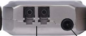
2 Strand LC-LC Fiber Optic Cable Input
