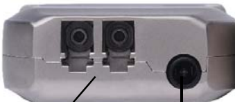
2 Strand LC-LC Fiber Optic Cable Input
