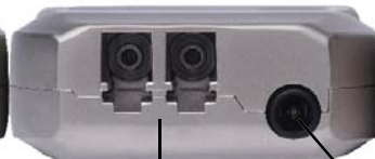
2 Strand LC-LC Fiber Optic Cable Input
