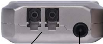
2 Strand LC-LC Fiber Optic Cable Input
