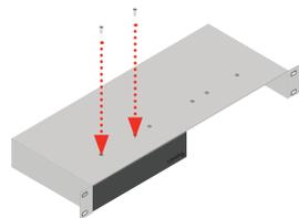
4. Ensure that unit has been installed securely in the rack tray.
