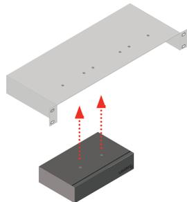
3. Install the two machine screws that are either provided with the product or need to be purchased separately.
