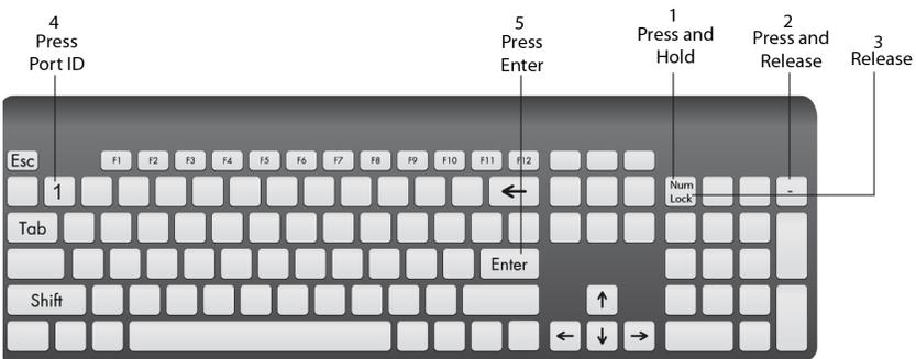
Repeat the steps using Port ID (1, 2, 3, 4) in step 4 to switch to the computer connected to that port. For more hotkeys, see *Hotkey Operation*, page 39.
