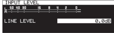
INPUT LEVEL screen when adjusting line level
