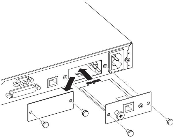
1. Remove the two screws from the plain panel and remove the panel itself.
