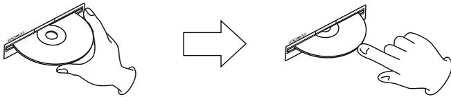
1. As shown in the illustration, hold the disc with the labeled side up and insert it part way into the slot.
