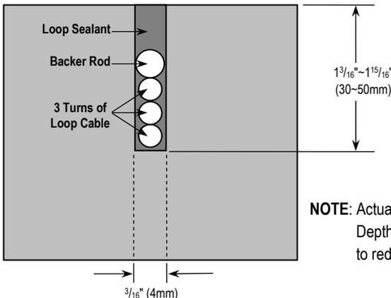
**NOTE:** Actual depth depends on number of loops. Depth may be less in concrete pavement to reduce potential for interference from rebar.
