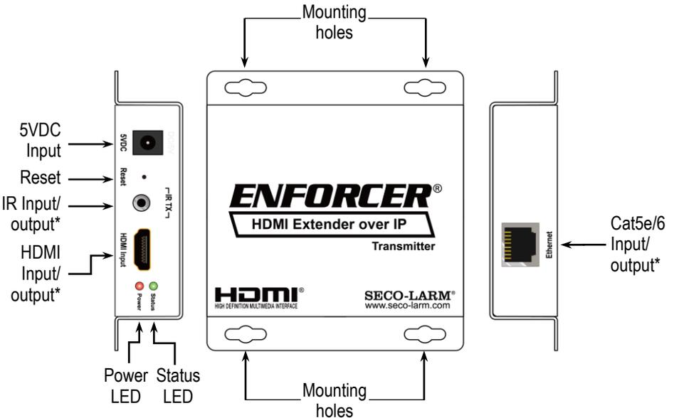
\*Input/output depends on whether the unit is a transmitter or receiver. A transmitter is shown above.
