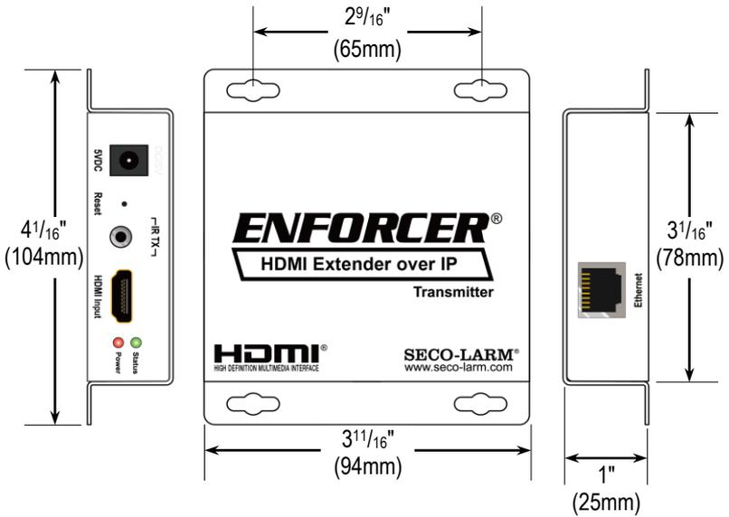
Note: The transmitter and receiver have the same dimensions.
