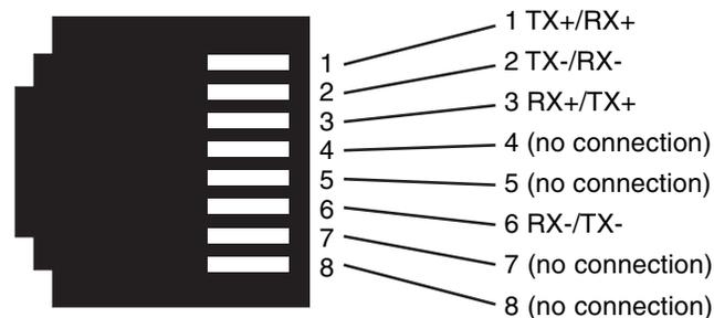
Figure 5. CL1214 10/100Base-T RJ-45 Connector Pin-out.
