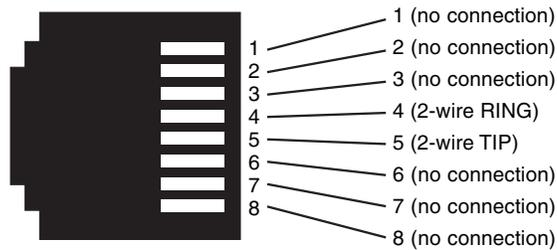
Figure 6. CL1214/S (RJ-45) POTS/ISDN interface.
