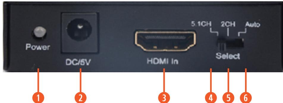
**① POWER AND ACTIVE LED:** With a bi-color LED, the light turns red when power adapter is connected and turns purple when starting to work.
