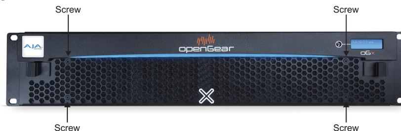
2. Using a Phillips screwdriver, remove the four screws that secure the faceplate. Set the screws aside.
