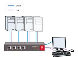
The switching section is hard wired to allow only one channel to be selected at any time. Common keyboard, mouse and video monitor are able to access multiple high security computers/networks, safe in the knowledge that data will not be transferred from one to another, either by user error or subversive attack.
