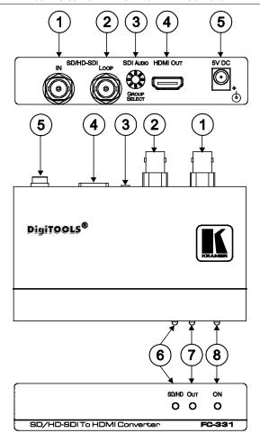
Figure 1: FC-331 SD/HD-SDI to HDMI Converter
