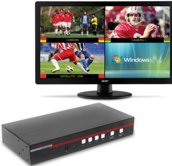
The SSW can display four Hi-definition sources on a single display and comes with pre-configured multi-view layouts (4 equal images as shown here, or one large and 3 smaller windows in various positions).
