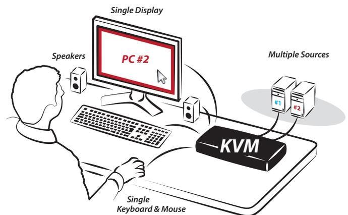
HSL Single-Head 2-Port KVM Switch System Diagram
