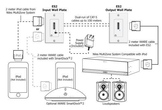
When not using a SmartDock2, use the cable included with your Niles MultiZone or control system. Caution: The 30-Pin Niles connector and 30-Pin iPod connector are not interchangeable. Attempting to force a mismatch may damage the connectors.
