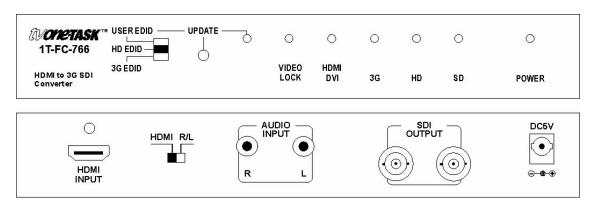
Connect the HDMI source device's output to the HDMI IN connector of the 1T-FC-766, using an appropriate high quality HDMI cable.
