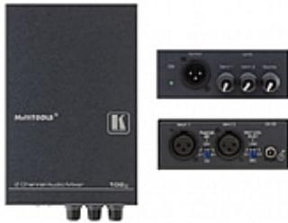
The **102xl** is a high-performance 2-channel mono audio mixer for line level and mic level balanced audio signals. The unit mixes two mono inputs and produces a mixed audio output signal.
