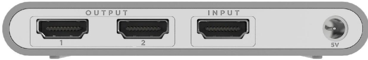
**1. HDMI OUT 1~2:** Using high-speed HDMI cables, connect each of the HDMI outputs from the SP-HD20-1X24K to an HDMI display for simultaneous HDMI distribution. You can also cascade the output to an HDMI transmitter to extend the operating distance.
