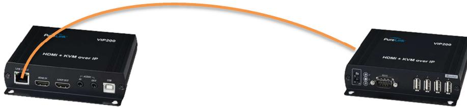
*Point to Point direct connection via CAT5e or better cable (Auto IP mode recommended)*
