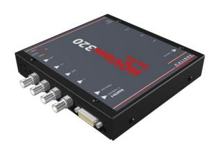
Harnessing the power of Reon™ video processor running state of the art HQV algorithms with expertly designed hardware and firmware from Calibre, HQView320 is a compact yet high performance image scaler with HDMI/DVI/Component/VGA input capability and HDMI/DVI output which provides stunning image quality for professional, broadcast and corporate AV users.
