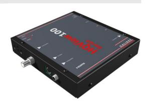
Harnessing the power of the Reon™ video processor running state of the art HQV™ algorithms with expertly designed hardware and firmware from Calibre, HQView100S is a compact yet high performance dedicated Composite and YC/S-Video image scaler which provides stunning image quality for professional, broadcast and corporate AV users.
